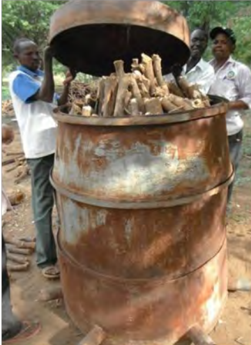
Portable metal kiln being loaded (left) and in use to make charcoal (right)
